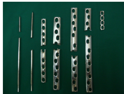
Figure II: Broken Schanz screws, dynamic compression plates and reconstruction plate.
